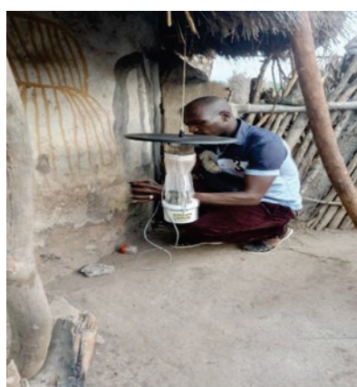
A CDC light trap outside a house
