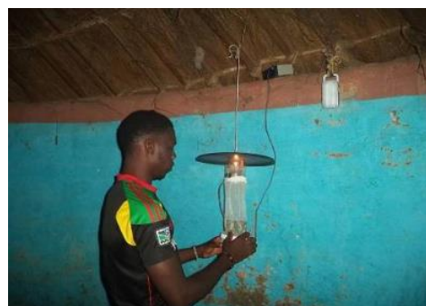
A CDC light trap placed outside to capture mosquitoes A CDC light trap placed inside to capture mosquitoes
