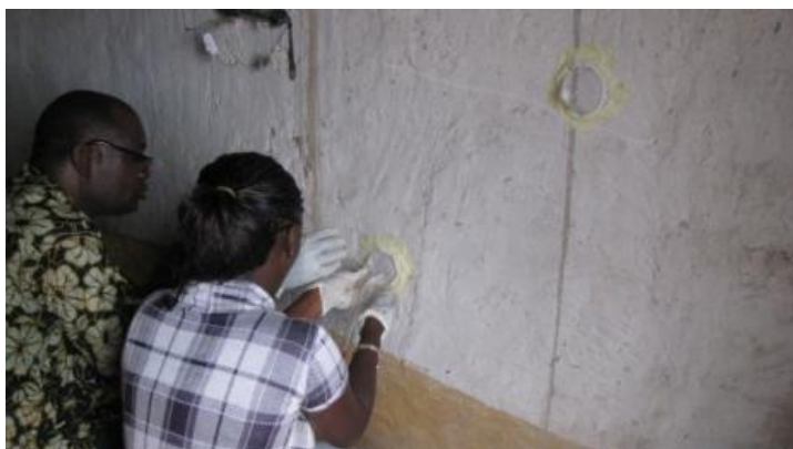
FIGURE 8: CONE TESTS ON A CEMENT WALL, KOULIKORO DISTRICT.
