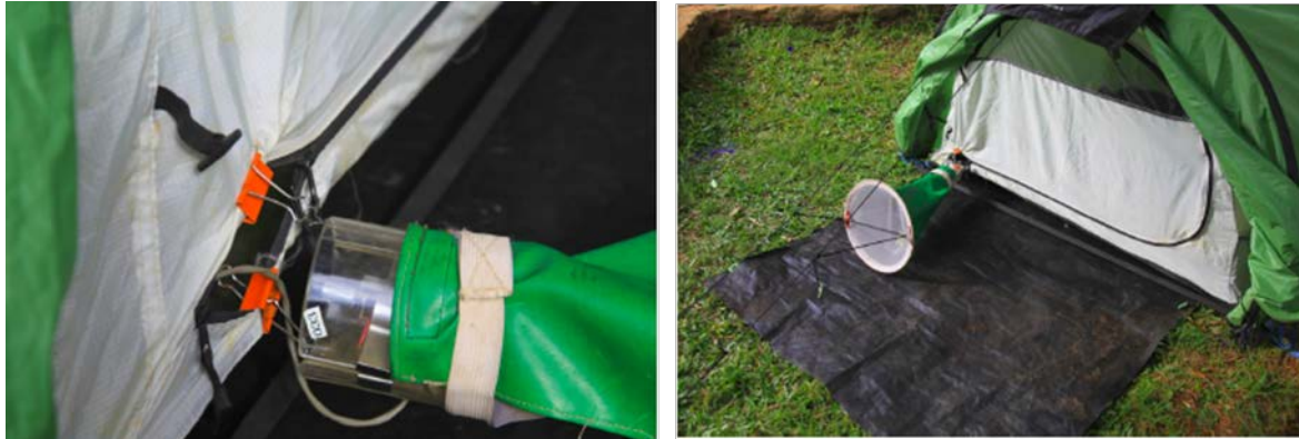
FIGURE 1: FURVELA TENT TRAP, SHOWING OPENING WITH CDC LIGHT TRAP (WITHOUT THE LIGHT) ATTACHED TO A SMALL OPENING.
