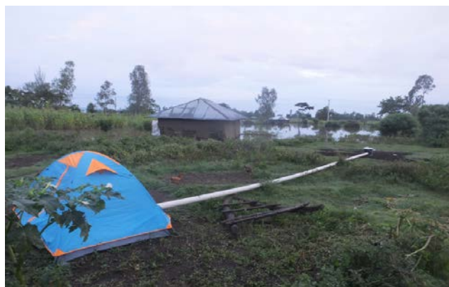
FIGURE 2: HOST DECOY TRAP, SHOWING HUMAN SLEEPING INSIDE TENT WITH TUBE TAKING HUMAN ODOR TO THE HEATING CYLINDER TRAP.
