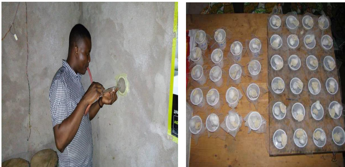
Figure 4. Exposure for 30 minutes to cement and mud walls treated with pirimiphos-methyl and mortality reading after 24 hours of observation
